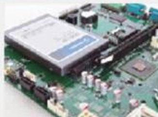
Direct HDD connection No internal cabling
