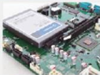
Direct HDD connection No internal cabling
